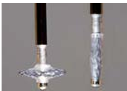
Fig. 4 – Deployed & Collapsed Disc
